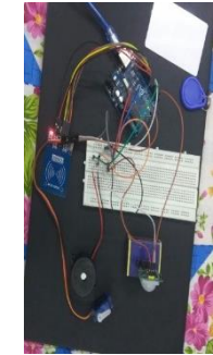
RFID – Alarm System
